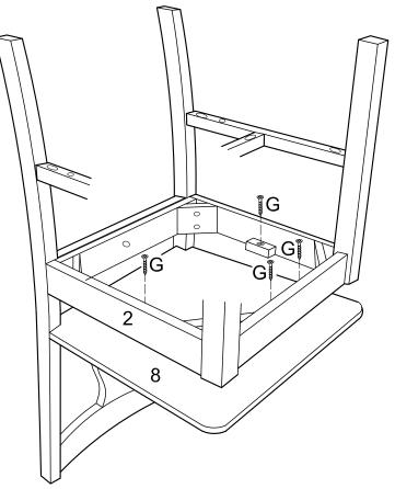
Attach seat (8) to seat frame (2) using screws (G). Tighten screws (G) with a screwdriver. Note: Seat (8) is not pre-drilled for screws (G) for added strength. Holes on seat bottom are not used for assembly.
