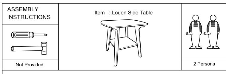
DO NOT fully tighten any of the bolts until the product is completely assembled, then put on a a flat surface to make sure the product is level and then fully tighten all the bolts.
