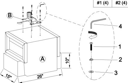
SHOWN ARE THE RECOMMENDED CHAIR SUPPORT DIMENSIONS FOR EASE OF BASE ASSEMBLY.
