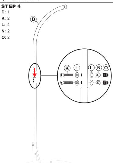
Slide Curved Pole (D) onto Straight Pole (C) and align the holes. Secure the poles using M10x50mm Bolts (K), Washer (L), and Lock Nuts (N) as shown. Place Large Hex Nut Caps (O) over the lock nuts.
