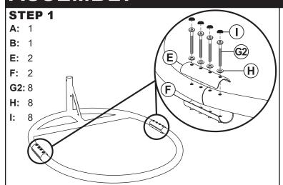
Align Base Back (A), Base Front (B), Top Base Connector (E), and Bottom Base Connector (F) and secure using Washer (H) and M6x50mm Bolts (G2). Place Bolt Caps (I) on the bolt heads.
