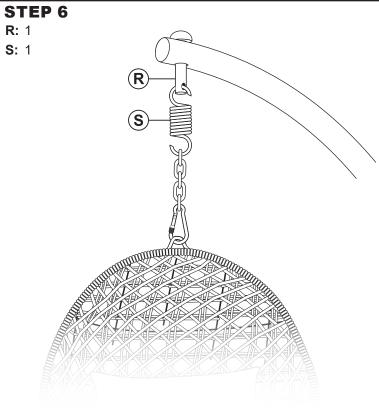
Place Pin (R) into the top of the curved pole. Insert Extension Spring (S) through the bottom of Pin (R).
