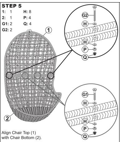
As shown, hand-tighten M6x50mm Bolts (G2), Washers (H) and Lock Nuts (P) to the outside mounting holes. Then, hand-tighten M6x45mm Bolts (G1), Washers (H) and Lock Nuts (P) into the center mounting holes.
