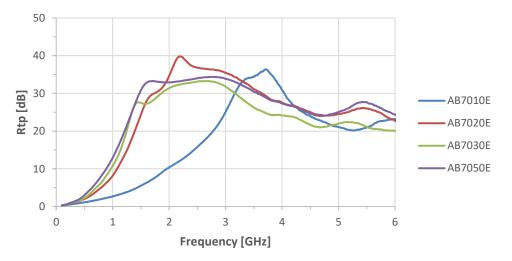
Transmision attenuation power ratio vs thickness
