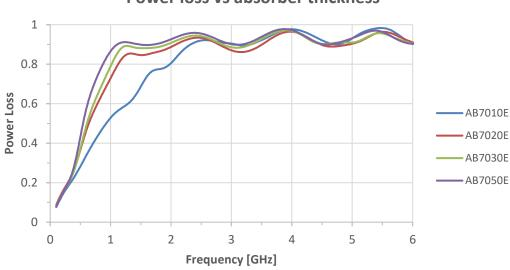
Power loss vs absorber thickness
