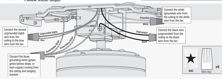
Ceiling Bracket Hanging Fan Wiring Motor Housing Blades Light
