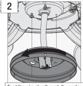
Feed the wire plug through the center hole of the upper switch housing, then wrap keyhole slots around the screws and twist counterclockwise.
