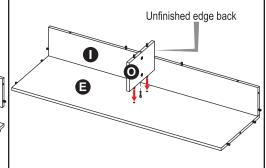
Ensuring the unfinished edge is facing the back panel, align Middle Panel (O) with Shelf (E) as shown.
