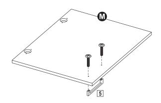
Ensuring the bolts install on the same side as the hinges, firmly fasten one Handle + 3/4" Screw (5) to Left Door (M).
