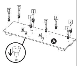
Install eight Spreading Bolts (2), and two Door Stops (6) into Bottom Panel (A) as shown.
