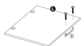
Ensuring the bolts install on the same side as the hinges, firmly fasten one Handle + 3/4" Screw (5) to Right Door (L).
