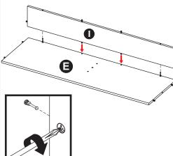
Ensuring the panels are installed facing the directions shown in the diagram, place Upper Back Panel (I) onto Shelf (E).
