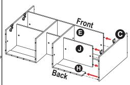
Align Shelf (E) with Left Middle Panel (F) and Right Middle Panel (G). Then, secure the cam locks.
