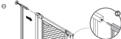
Connect the extension frames to gate frame by inserting the pins on the extension frames into the holes in the gate frame.
