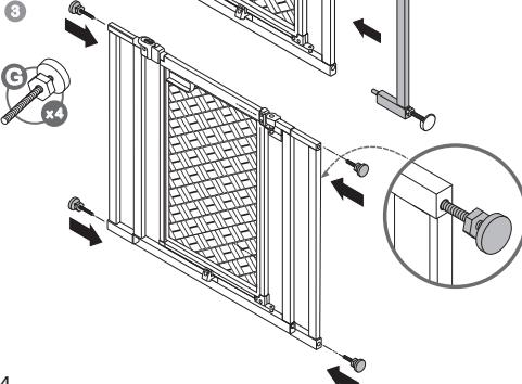
Slide tension bolts into upper and lower holes on both sides of the gate assembly. The holes are not threaded and that the tension bolts should slide freely.
