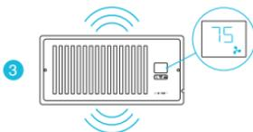
When the probe detects the airflow temperature has fallen below your **Cooling Trigger**, it will activate the fans.
