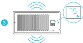
When the probe detects the airflow temperature has risen above your **Heating Trigger**, it will activate the fans.
