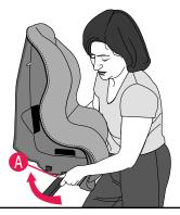
Lift the child restraint and flip the recline stand (A) toward the rear, as shown, to the *upright* position.
