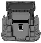
**Note:** if you are using the buckle in the front slot and need to shorten it, pull it down and then push the anchor up through the rear slot and make sure the anchor is flush with the surface of the seating area.
