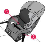
When the buckle strap () is in the rear slot, route aircraft seat belt (A) in front of the buckle strap, as shown.
