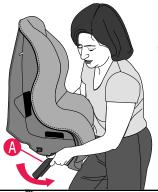
Lift the child restraint and flip the recline stand (A) toward the front, as shown, to the *recline* position.
