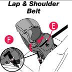
Pull the seat pad off of the front of the child restraint. Route the vehicle seat belt • through the rear-facing belt path •, continue through the opposite opening of the child restraint. Fasten the vehicle seat belt, as shown, depending on your type of seat belt.
