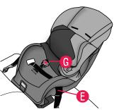
When the buckle strap (s) is in the **rear** slot, route Lower Anchor Connector strap (s) in front of the buckle strap, as shown.
