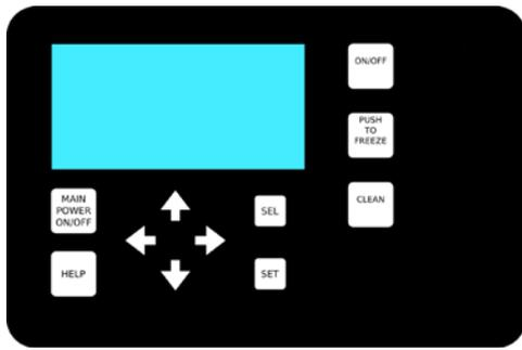
**Figure 3-2 IntelliTec2™ Control**
