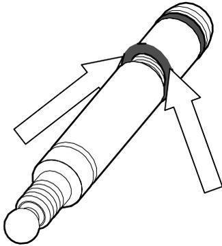
**Figure 3-4 Removing O-Ring**
