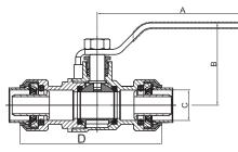
Not for use with PEX-AL-PEX or PEX tubing with an oxygen barrier. NOT FOR USE AT OR BELOW GROUND LEVEL.
