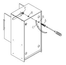
Step 2 Use 1/4" (6.5 mm) drill bit to drill hole in wall
