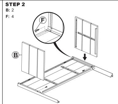
Align two End Panels (B) with the legs of one assembled side panel. Secure each side panel using two M4x12mm Screws (F).
