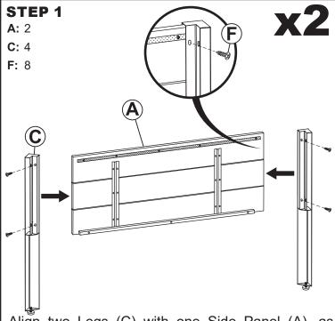
Align two Legs (C) with one Side Panel (A), as shown. Align the indents on Panel (A) with the mounting holes in the legs, secure each leg using two M4x12mm Screws (F).
