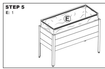
Install Planter Bag (E) into the planter box by aligning the hook and loop fastener strip on the bag to the strip inside the planter box.
