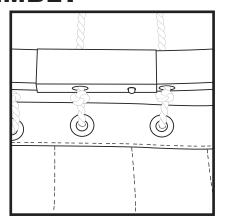
Push the bars together until the spring button snaps through the hole in the metal bracket.
