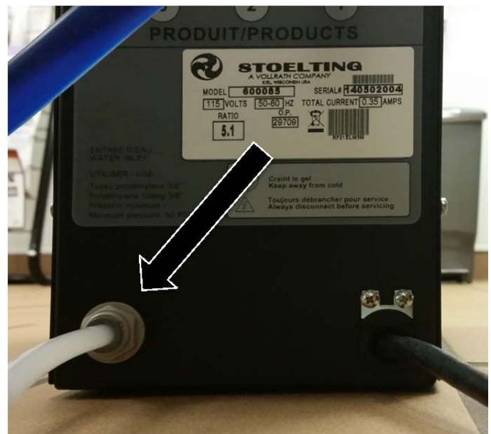
Water Supply Connection
