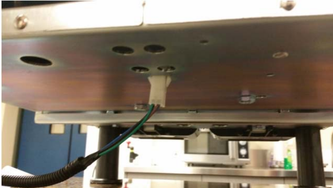
Connect Wiring to Bottom of Machine
