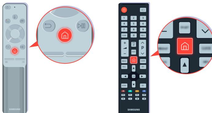
If there is sound but it is not clear, run a diagnostic test. On the remote control, press the
