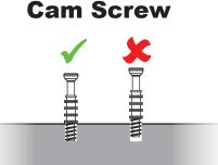
Use a screwdriver to tighten the cam screw until the shoulder is flush with the panel. Do not overtighten or under-tighten.
