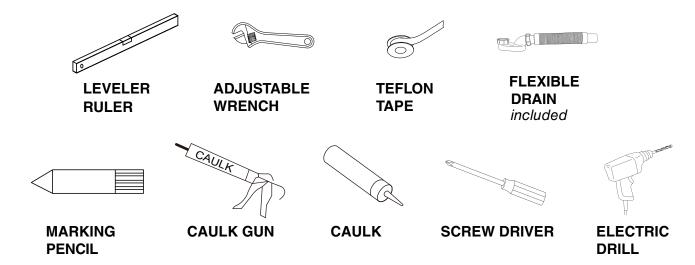
**NOTE:** THE INCLUDED FLEXIBLE DRAIN IS TO BE USED ONLY TO TEST THE BATHTUB BEFORE PERMANENT INSTALLATION. IT IS THE RESPONSIBILITY OF THE INSTALLER TO PROVIDE THE PERMANENT DRAIN ASSEMBLY.
