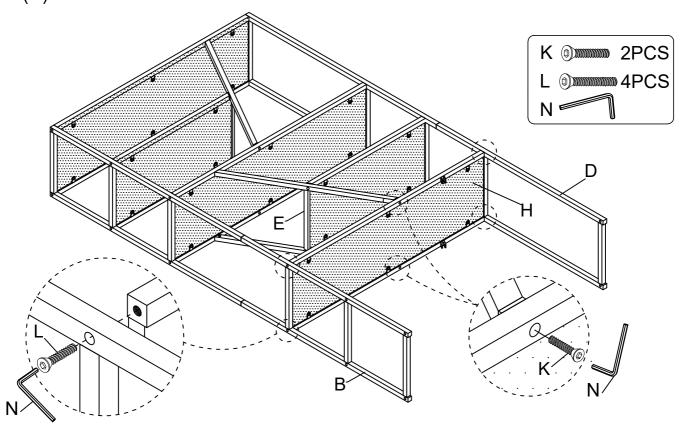
Insert the rest 1pc Shelf Frame (E) to the Shelf Board - Long (H), using Bolt (J) & Flat Washer (M) to fasten by Allen Key (N).
