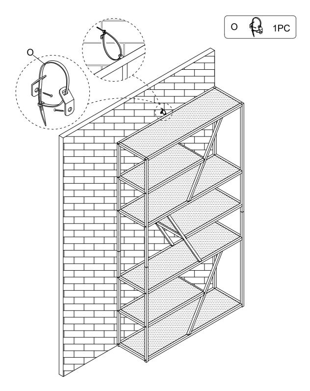
Adjust any parts out of alignment and tighten all bolts and screws from steps 1 through 12.
