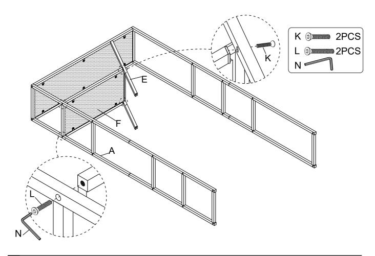
Assemble 1pc Shelf Board - Long (H) to Left Top Frame - Short (A), Shelf Frame (E) and Right Top Frame (C), using Bolt (K) & Bolt (L) to fasten by Allen Key (N).
