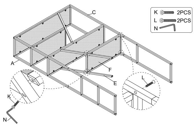
Assemble the rest 1pc Shelf Board (H) to Left Bottom Frame (B), Shelf Frame (E) and Right Bottom Frame (D), using Bolt (K) & Bolt (L) to fasten by Allen Key (N).
