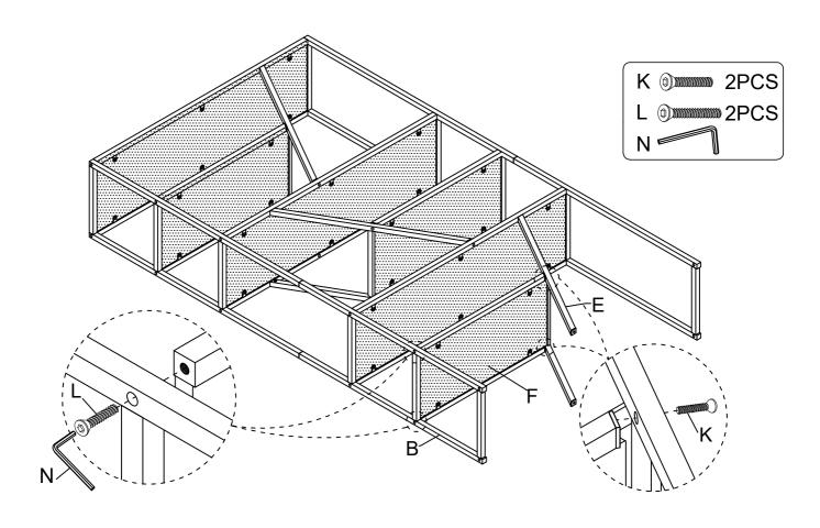
Assemble Bottom Panel (I) to Left Bottom Frame (B), Shelf Frame - Short (E) & Right Bottom Frame (D), using Bolt (K) & Bolt (L) to fasten by Allen Key (N).
