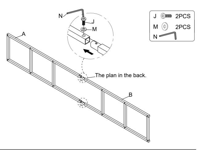
2 Insert Right Bottom Frame (D) to the Right Top Frame (C), then using Bolt (J) & Flat Washer (M) to fasten by Allen Key (N).
