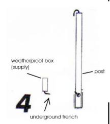
Make power connection through a weatherproof box and run line through trench to lamp post hole. Feed line from the inlet hole at post base to the top of the post.
