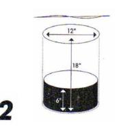
Dig a hole 12" diameter by 18" deep. Fill in 6" with gravel.
