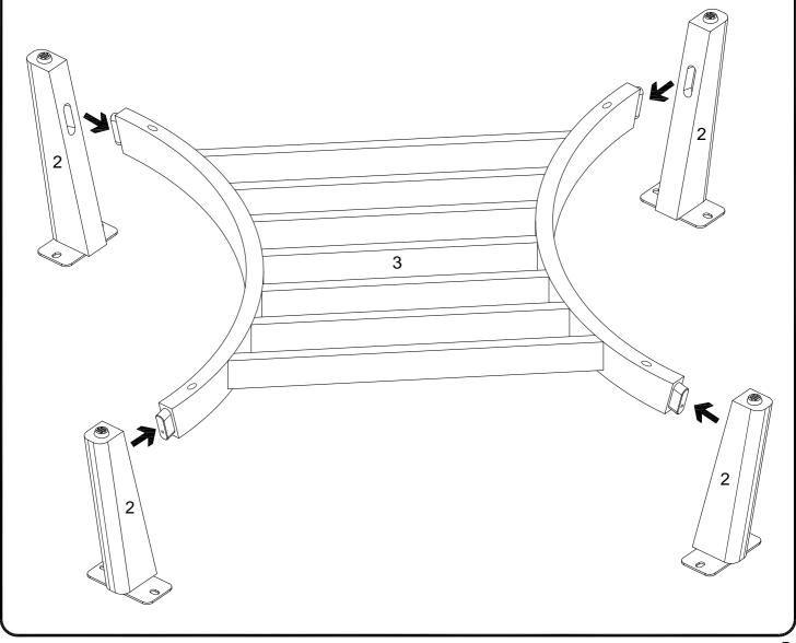
Flip the Seat Cushion (1) over and place the frame you just made on the bottom. Line up the Legs (2) with the holes and secure everything using a Washer (C), Spring Washer (B), and Bolt (A).
