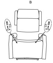
STEP 1 - Place Bracket into Sleeve and press top of back down firmly to lock your KD back in place
