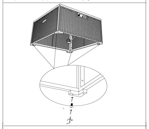
4.Connect adjust foot (P) to the botom of fire pit using 8pcs screws (Q) And tighten the Bolts.
