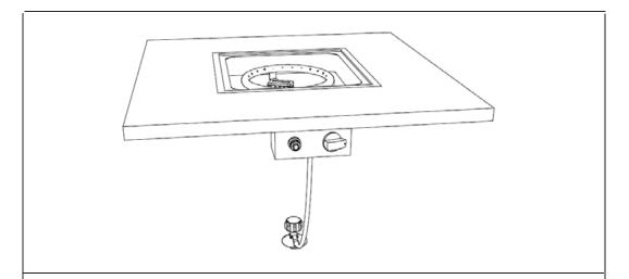
1. Check the control knob for gas supply system is turned to OFF position before starting your assembly.
