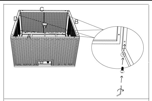
3. Connect panel (A,C) with Panel (B,D) together using 8pcs screws (K) and 8pcs M6 washer(M) . Please do not fully tighten.
