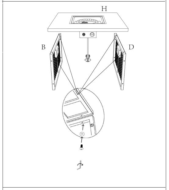
2. Connect panel (B,D) to the table top (H) by 4pcs screws (K) and 4pcs M6 washer(M). Please do not fully tighten.
