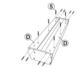
Secure two Shelf Backboards (D) to the back of the shelf boards using six M3.5x30mm Screws (5).
