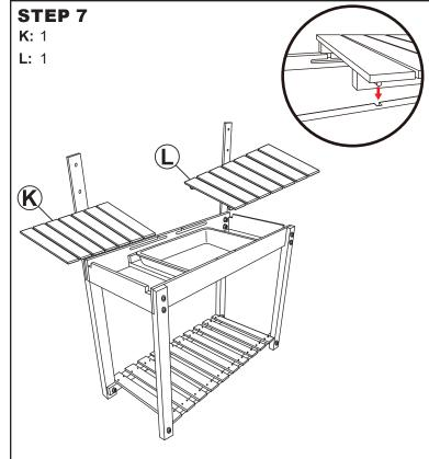
Insert the dowels under Left Tabletop (K) and Right Tabletop (L) into the grooves in the table frame.
