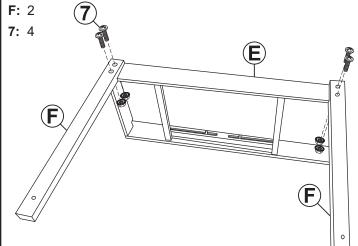
Secure two Front Legs (F) to Table Frame (E) using four M6x45mm Bolt Sets (7).
