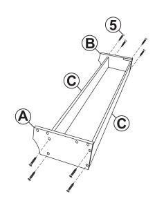
Firmly secure Right Shelf Panel (A) and Left Shelf Panel (B) to two Top Shelf Boards (C) using eight M3.5x30mm Screws (5).
