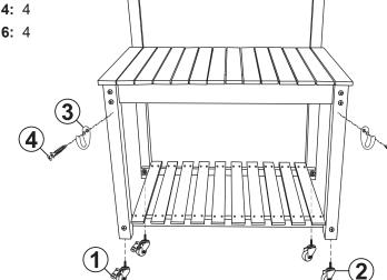
Secure the top shelf to the shelf supports using four M6x25mm Bolts (6).
