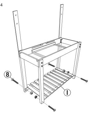
Secure Bottom Shelf (I) to the legs using four M6x60mm Bolt Sets (8).
