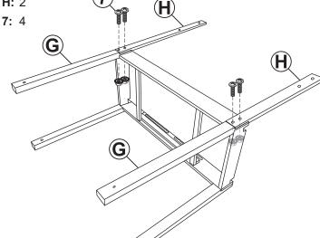
As shown, secure two Back Legs (G) and two Shelf Supports (H) to the back of the table frame using four M6x45mm Bolt Sets (7).
