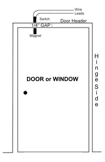
Attach switch to header or side of door or window frame (NOT on hinge side)
