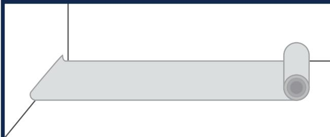
The subfloor must be dry, fully cured, and free of hydrostatic pressure. See instructions below regarding moisture testing your subfloor. A moisture barrier such as 6mil plastic or CALI Complete may be necessary. Make sure the subfloor is flat, clean and free of debris.
