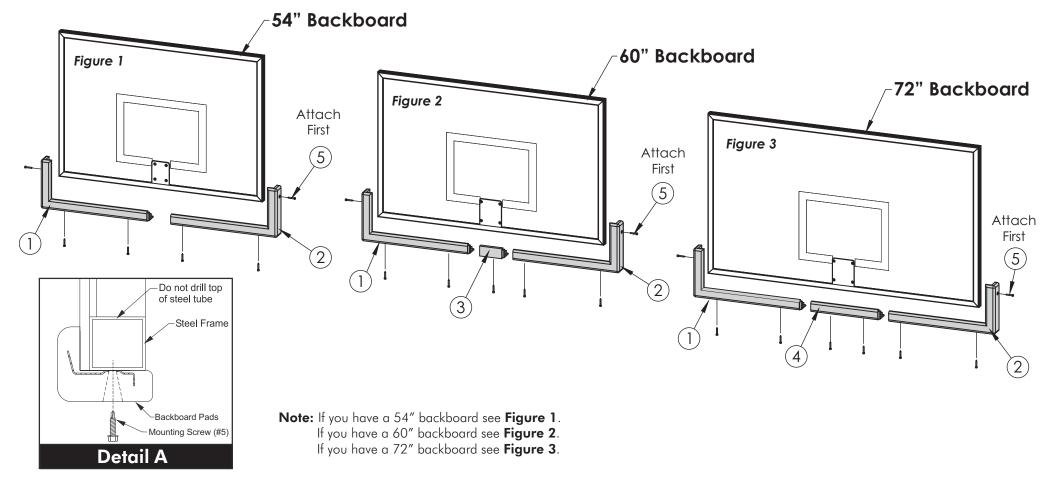
1. Use the Backboard Pads as a Template and mark the hole locations on the backboard frame.
