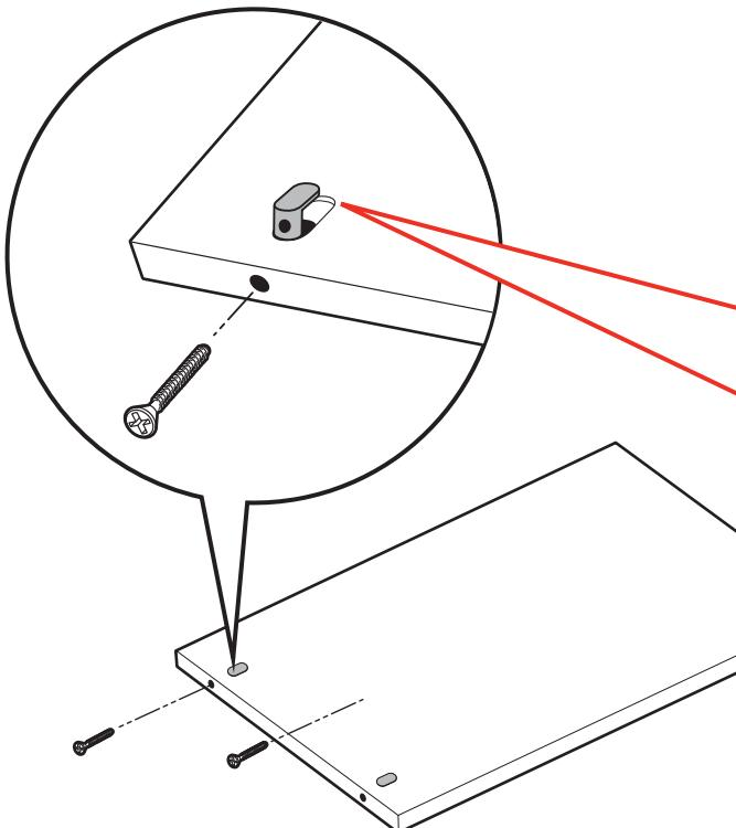
**en** **IMPORTANT:** Barrel nuts and screws are used to join the main wood panels together. The pre-installed barrel nuts have been properly aligned at the factory to allow the screws to easily join the panels.
