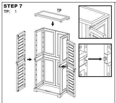
Ensuring the pivot pins on the top doors align with the front of Top Panel (TP), firmly press the top to secure it to the unit.
