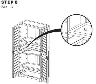
Insert Shelf (SL) into the unit at a slight angle and align the shelf with one side of the unit. Then, gently press on the opposite side of the shelf until the shelf locks into place.
