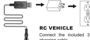
Connect the included 3.7V battery to the charging cable.
