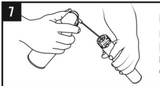
**Remove excess water and fouling with compressed air and / or shooting several rounds (supersonic is recommended) through the suppressor to eject the loosened fouling.**
