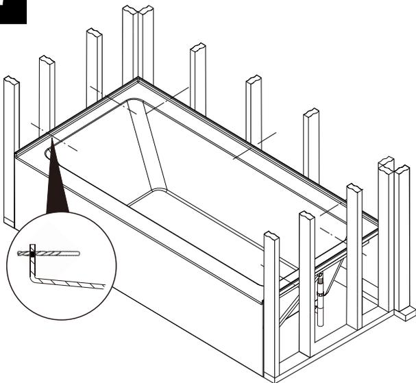
Drill 3/16" clearance holes in flat area of top flanges, and centered on each stud. Evenly space holes on front vertical flanges.
