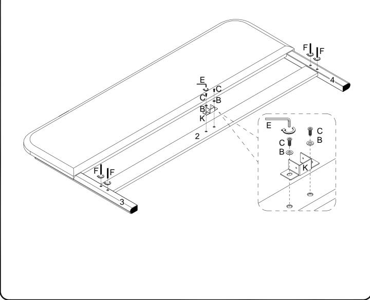
Attach the other U bracket (K) to the Bottom Rail (6) using the using the same Flat washers (B) and Bolts (C).
