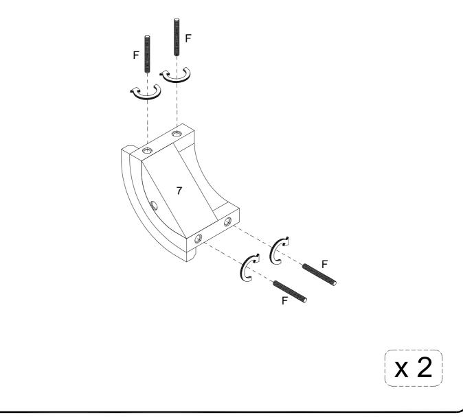
After removing the plastic caps on the Legs (8), twist them into the bottom of the Curved Corner Pieces (7) until tight.
