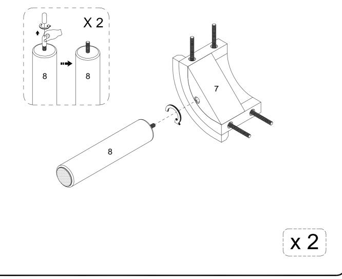
Remember how we put the Headboard together? Follow that same process and a ttach the Curved Corner Pieces (7) to each side of the Bottom Rail (6) using the Half-moon washers (G) and Nuts (H) tightening with the Wrench (J).
