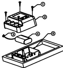
▪ Remove the screws (part 1) from the control panel cover (part 2) using a Phillips-head screwdriver.
