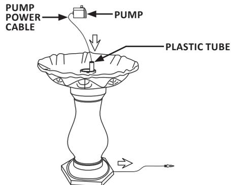
**3.** Attach the pump to the hose in the fountain body. Place the fountain body on the reservoir and twist the ornate column to secure.
