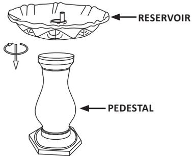
**2.** Feed the pump power cable through the plastic tube in the reservoir, and through the channel on bottom of the pedestal.
