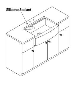
STEP 6 Install drain, trap, water supply and faucet according to manufacturer's instruction. Run water into sink and check for leaks
