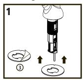
Locate the adhesive gasket ③. Remove the liner from the top of the adhesive gasket and affix to the bottom of the dispenser. Remove the liner from the bottom of the gasket.
