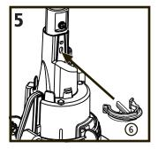
Secure the bottle support to the dispenser assembly by pushing the retaining clip (6) into place.
