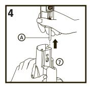
Align the metal rod (A) from threaded shank with small guide hole in the bottle support (7). Slide the bottle support up onto the rod.
