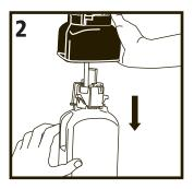
While still pushing the latch release, pull downward on the bottle and remove it from the bottle support.
