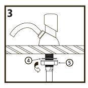
From underneath the counter, secure lock washer (4) and mounting nut (5) and tighten to underside of counter.
