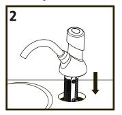
Position the dispenser assembly by guiding the threaded shank through the hole in the counter. Make sure the spout is facing into the sink bowl. Press down firmly on dispenser assembly to ensure it is securely attached to counter.
