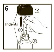
Refill Installation (refill sold separately) Feed the dispense tube (B) on the refill bottle (B) through the bottle support (D), aligning the two indents. Slide the refill upward until it snaps into place.
