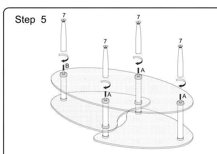
Screw legs (7) onto all rods (A,B). Ensure that legs (7) fit snuggly into the decorative rings placed in the previous step.
