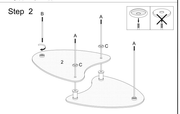
Slide top glass (2) then decorative rings (C) onto middle rods (A). Screw short rod (B) into the open plate of top glass (2).
