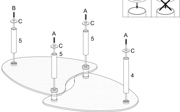
Slide cylinder (4) onto right long rod (A). Slide cylinders (5) onto middle long rods (A) and short rod (B). Slide decorative rings (C) onto all rods (A,B). Snap decorative rings (C) onto cylinders (4,5).
