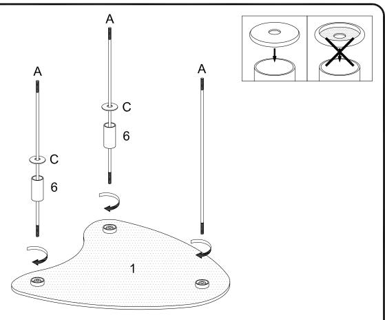
Carefully lay top glass (1) up-side-down on a soft surface. Screw long rods (A) into the plates of top glass (1). Slide cylinders (6) and decorative rings (C) onto middle long rods (A). Snap decorative rings (C) onto cylinders (6).
