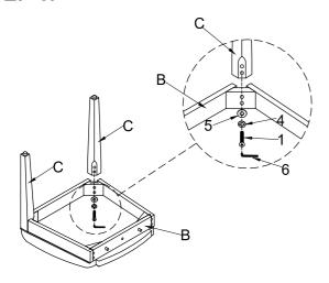
DO NOT TIGHTEN BOLTS COMPLETELY
