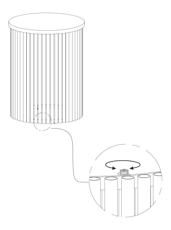
Note: Levelers on bottom of base can be adjusted if floor is uneven.
