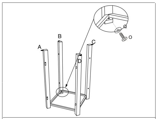
1. Connect the tank holder/base (I) With table Lets(A/B/C/D) by 4pcs screws (O) and 4pcs M6 washers(Q).
