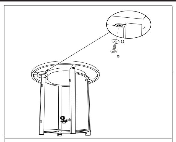
3.Attach the assembled base to the bottom of top using 4pcs of screws (R), and 4pcs M6 washers(Q), make sure the panel (L) faces the valve stem. Tighten all screws.
