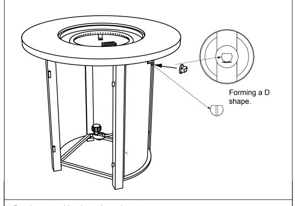
4. Put the control knob on the valve stem.
