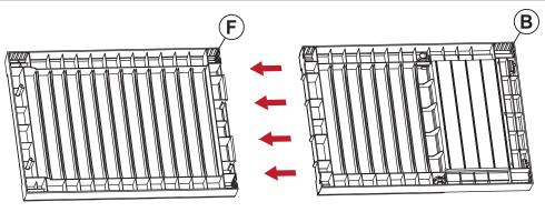
Connect Rear Seat Panel (B) into Front Seat Panel (F).
