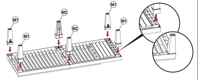
Install four Corner Legs (M1) and two Middle Legs to the underside of the seat panel, as shown.
