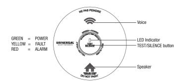
The device provides voice messages, in addition to audible alarms, to alert you of smoke or carbon monoxide detection
