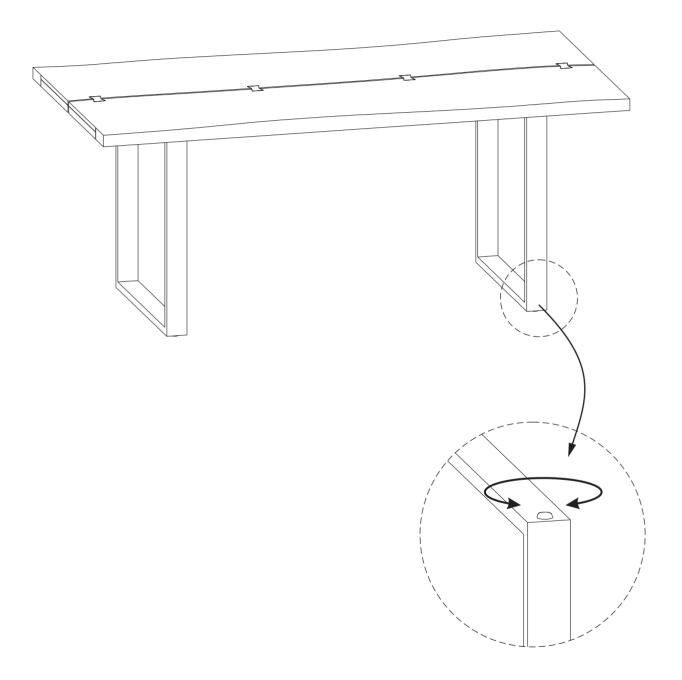
**Note:** Levelers on bottom of legs can be adjusted if floor is uneven.
