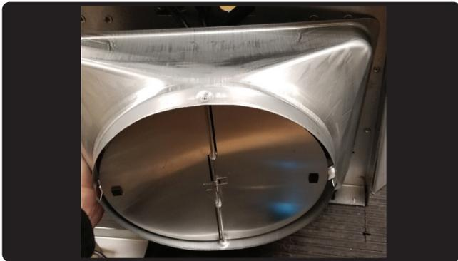
9. Attach 10" round blower collar on top of the hood body by (4) M4x8 screws.
