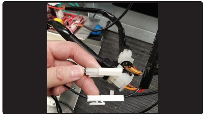
12. Thread both blower wires through the hood body wiring holes. Connect the 9-pin blower plugs and black single pin power cables together from both blowers.
