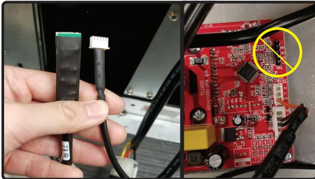
15. Connect the 5-pin white male connector from PBD-1300B control board to the 5-pin female connector leading from the range hood's switch assembly. Do not connect the 5-pin female connector to the PBD-1300B control board.
