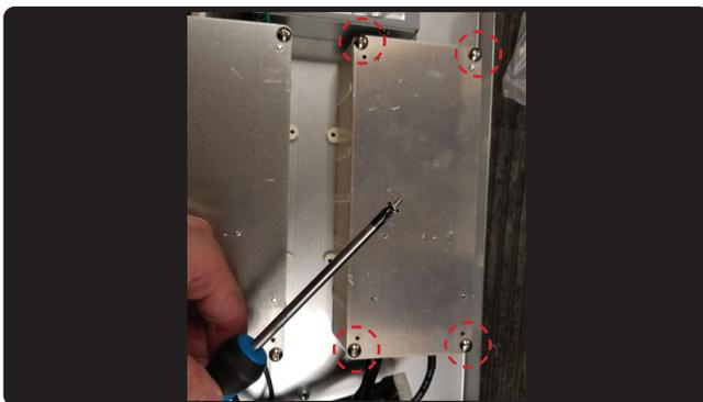
17. Secure both control boards back to the component box by (4) screws each.
