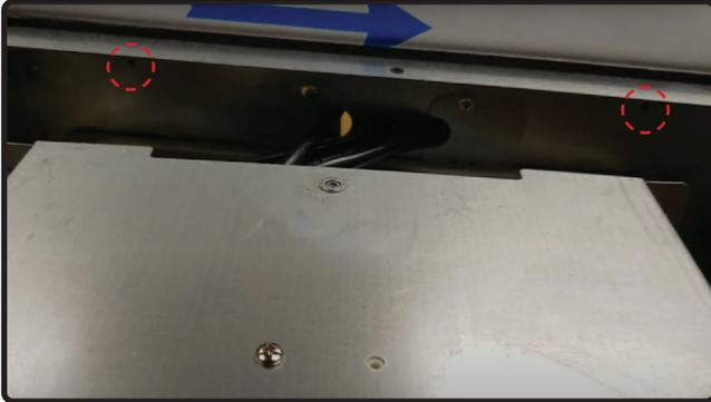
19. Secure the electrical bracket to hood body by (2) screws.
