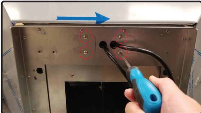
3. Remove both wiring hole covers by (2) screws each.
