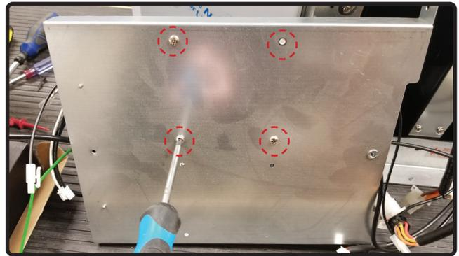
10. Secure PBD-1300B component box to electronics bracket by (4) screws.
