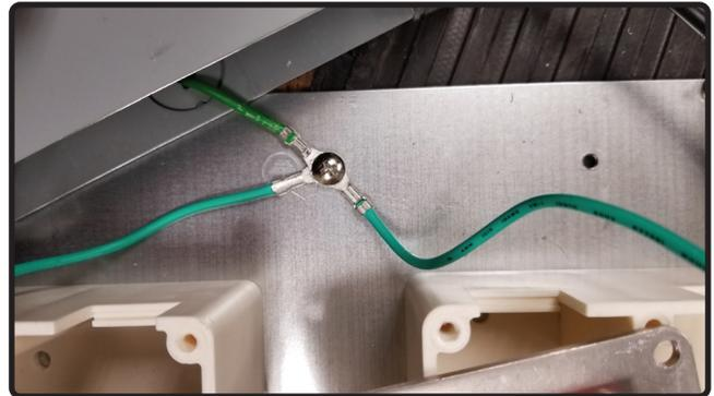
16. Secure the (3) ground wires together by (1) screw. The ground wires are from the electrical box and each control board.
