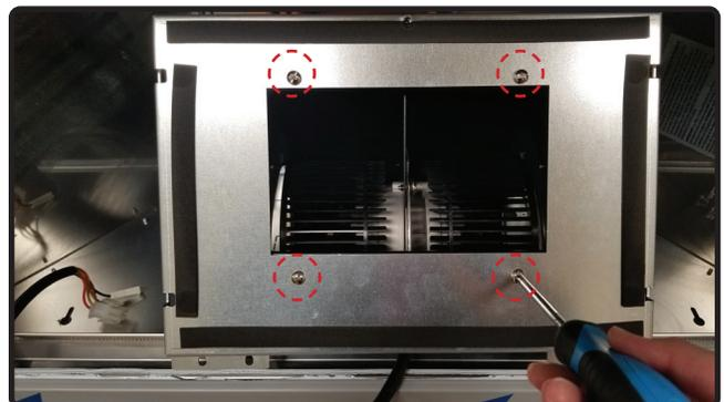
6. Remove (4) screws attaching single blower to single blower plate.
