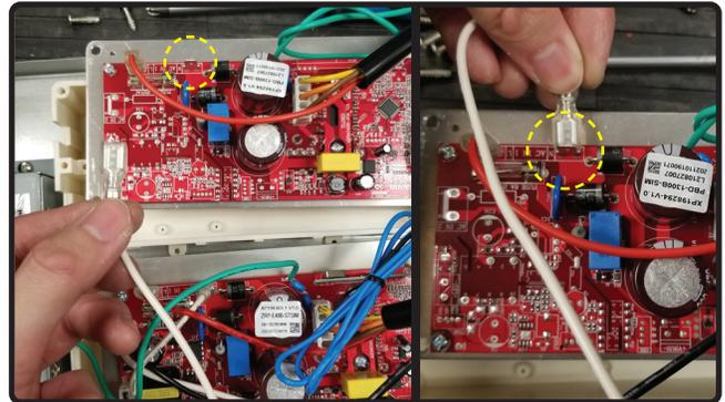
14. Locate loose white power wire with female spade connector from the main control board and attach it to the PBD-1300B control board.
