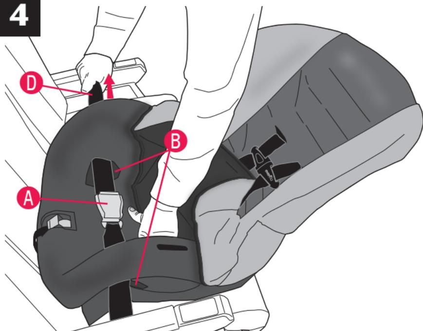
The aircraft seat belt **A** must be as tight as possible. Route the excess seat belt strap **D** back through the rear-facing belt path **B** opening, as shown above. Using your full weight, push the child restraint firmly onto the aircraft seat while pulling on the excess seat belt strap to tighten.
