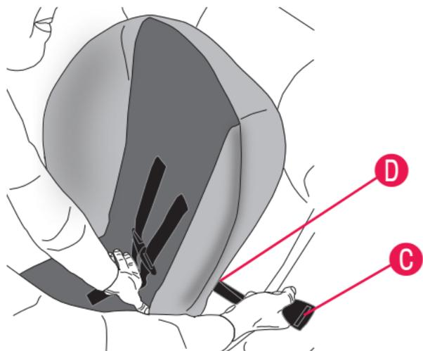
The aircraft seat belt must be as tight as possible. Route the excess aircraft seat belt strap **C** back through the forward-facing belt path **D** opening, as shown above. Using your full weight, push the child restraint firmly onto the aircraft seat while pulling on the excess seat belt strap to tighten.
