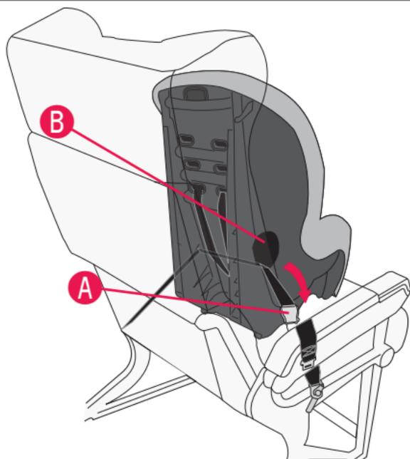
Route the aircraft seat belt **A** through the forward-facing belt path opening in the back of the child restraint and continue through the belt path opening **B** on the opposite side of the child restraint.
