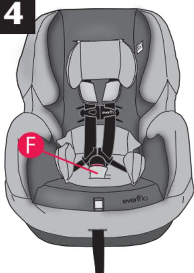
To remove the buckle cover **F**, press the red buckle release under the buckle cover, and remove buckle tongues. Pull buckle cover off the buckle.
