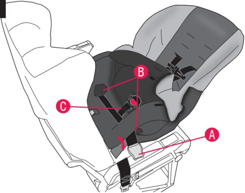
Pull the seat pad off the front of the child restraint. Route the aircraft seat belt **A** through the rear-facing belt path **B** opening on one side and continue through the belt path opening on the opposite side of the child restraint, as shown above.
