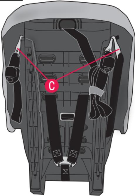
When the Lower Anchor Connector assembly is not in use you **MUST** attach the hooks **C** to the back of the child restraint. A loose Lower Anchor Connector assembly strap and hook may injure your child.
