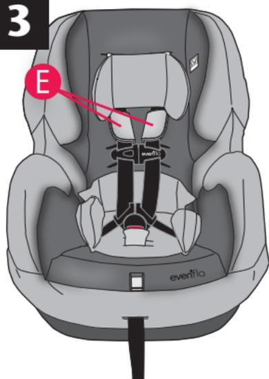
To remove the harness covers **E**, follow steps for Positioning the Harness Strap (p. 36). After Step 2, slide harness covers off harness straps. Continue with Step 3.
