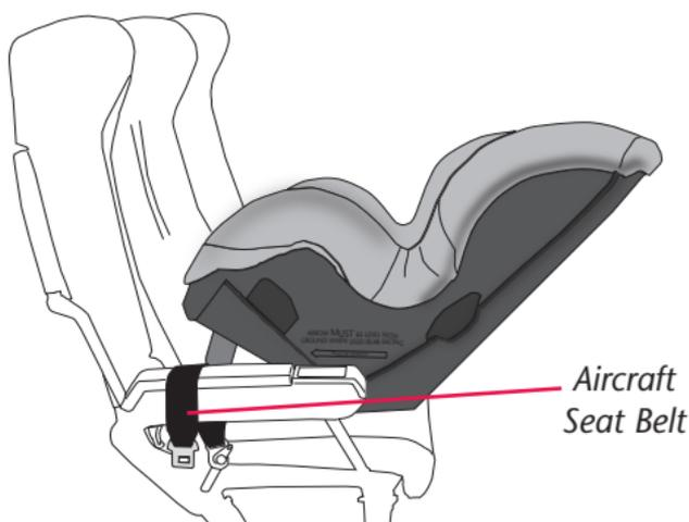
Adjust the child restraint to its **recline position** (page 38), then place it on the aircraft seat **rear-facing**, as shown above.
