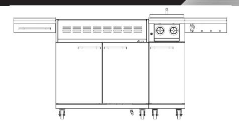
FRONT VIEW, shown with grill head removed Side shelves extended Optional side burner cart installed (XOGCARTSBXLT) GRILL + CART DIMENSIONS
