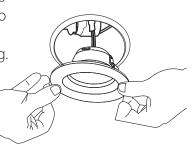
6 Carefully route wires into housing and push the downlight upward making sure it is flush to the ceiling surface.
