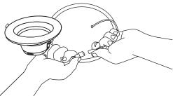
4 If using an incadescent housing, screw the edison base socket string into the socket. Mate the downlight connector into the Edison (or GU24) base
