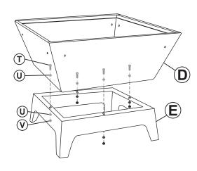
Align Fire-Bowl (D) with Base (E) and secure using four 1/4"x5/8" Bolts (T), eight Washers (U), and four Nuts (V), as shown.
