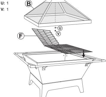
Attach Screen Handle (A) to Spark Screen (B) using one Washer (U) and one Nut (V).
