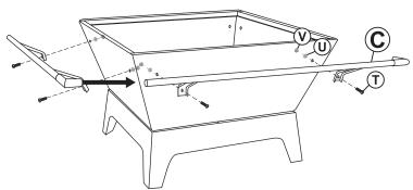
Loosely secure one Top Ring (C) to the fire-bowl by hand tightening one 1/4"x5/8" Bolt (T), one Washer (U), and one Nut (V), as shown.
