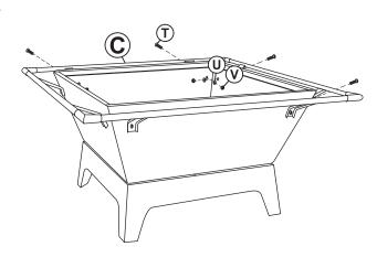
Align two Top Rings (C) with the loosely installed rings and secure using four 1/4"x5/8" Bolts (T), four Washers (U), and four Nuts (V).
