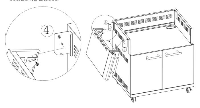
To attach the Right Side Shelf Front #(20) to the Right Side Shelf #(21), turn both parts upside down. Start, but do not tighten down 2 - M5x10 bolts as shown below into the Right Side Shelf Front #(20). Align the heads of the bolts with the keyhole slots in the Right Side Shelf #(21) and slide into place to align both parts. Install the additional 3 - M5x10 bolts as shown and tighten all 5 bolts.
