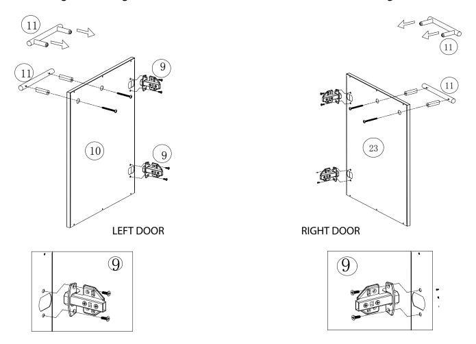
Attach the Left Door / Hinge Assembly to the Cart Left Side #(12) with 8 - M4x12 screws. Attach the Right Door / Hinge Assembly to the Cart Right Side #(24) with 8 - M4x12 screws.
