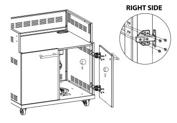
To adjust the gap between the doors - turn Screw A on the hinges.
