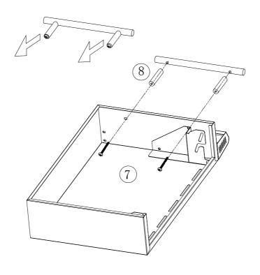
Install an M5x15 shoulder bolt at the top of each Shelf Bracket #(4, 5). After the installation use an additional M5x15 shoulder bolt to install the Side Shelf Assembly to the Shelf Bracket, front and rear as shown.
