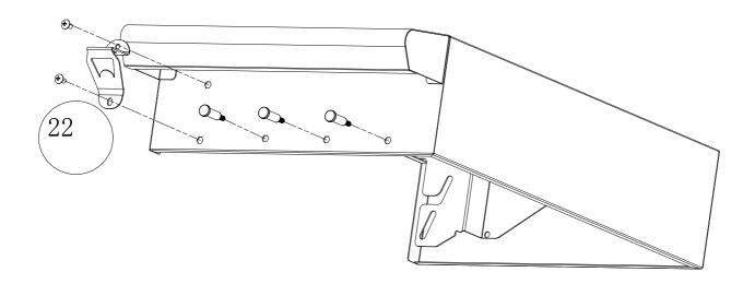
Install an M5x15 shoulder bolt at the top of each Shelf Bracket #(4, 5). After the installation use an additional M5x15 shoulder bolt to install the Side Shelf Assembly to the Shelf Bracket, front and rear as shown.
