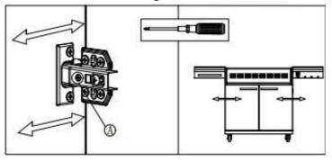
To adjust the gap between the door and the frame - turn Screw B on the hinges.
