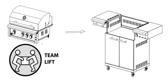
OPEN THE GRILL AND REMOVE THE GRATES TO REDUCE ITS WEIGHT.
