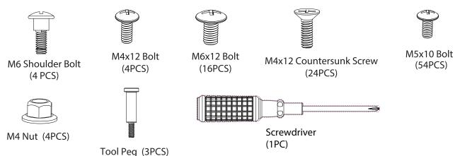
Use 16 - M6x12 bolts to install the Casters onto the Base Plate #(16) There are two caster types, one with locks and one without. First install the casters without locks #(17) and then the casters with the locks #(19). Make sure the Locking Casters are located on the left hand side.
